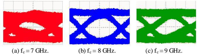
Fig. 8. Measured eye diagrams at 2.5 Gbps. The input power is -6 dBm. 20 mV/div; 100 ps/div.
