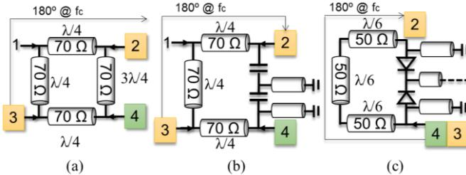
Fig. 2. Schematic of conventional rat race [3] (left); rat race with high-pass compensation [14] (middle); and this work (right).
