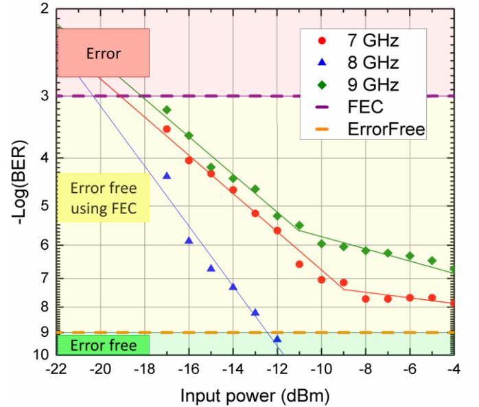
Fig. 7. BER curves versus input power at 2.5 Gbps.
