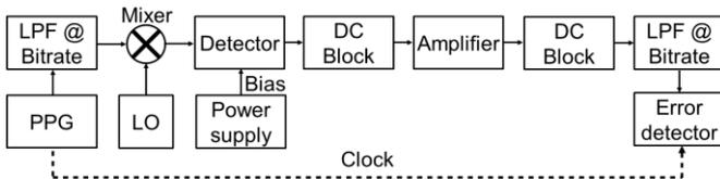
Fig. 6. Set-up used for measuring the bit error ratio, BER.
