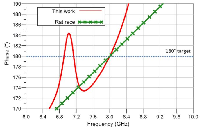
Fig. 3. Comparison of phase balance bandwidth between a rat race (green, cross) and this work (red).
