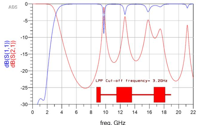
Fig. 4. S-Parameters of the low pass filter (LPF).
