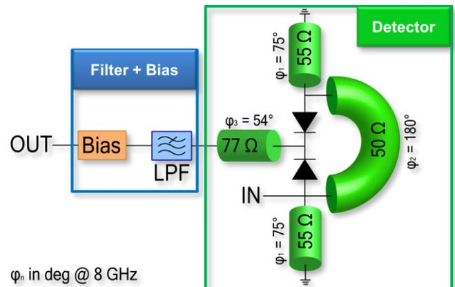
Fig. 1. Schematic of the proposed detector circuit.
